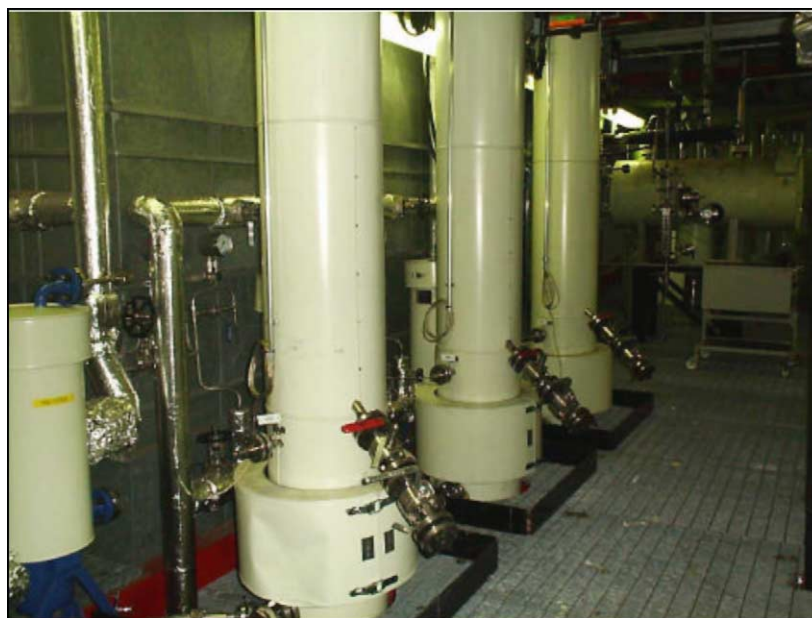
Fig. 5. Reactor section of AlkyClean SM demonstration plant.
